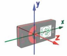
During the source search it is essential to analyze the instant values along individual axes for the purpose of source direction identification
